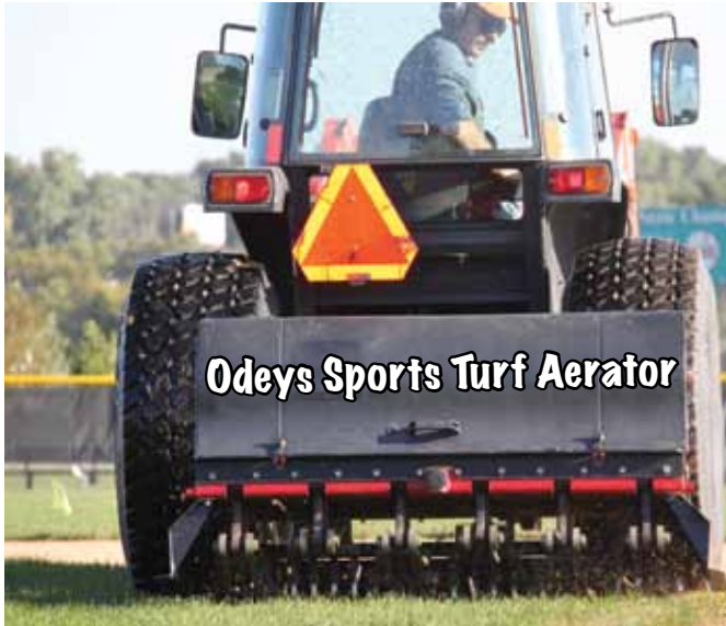
Holes on a 2" x 2" grid = 36 per square foot
